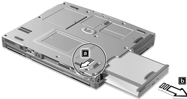
5. Insert a drive module into the AcerMedia drive bay. The bay release latch locks it in place.
