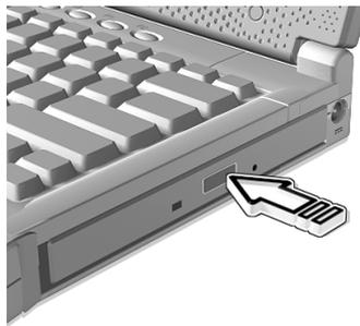
When the power is off, you can eject the drive tray using the emergency eject hole. See page 48.
