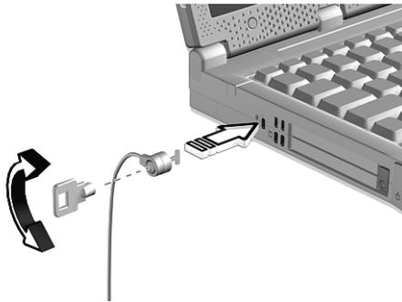
Wrap a computer security lock cable around an immovable object such as a table or locked drawer handle. Insert the lock into the notch and turn the key to secure the lock.
