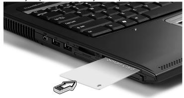
To remove the SmartCard first press the SmartCard (a) and remove the SmartCard (b) as shown in the illustration below.
