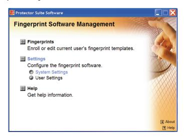
Once the System Settings window opens, click the TPM tab to access controls for your system's TPM module.
