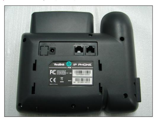
Step2: Loosen 6pcs of screws, open the back shell.
