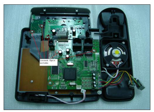
**Step5:** Loosen 4pcs of screws on the LCD module and take away the damaged one.
