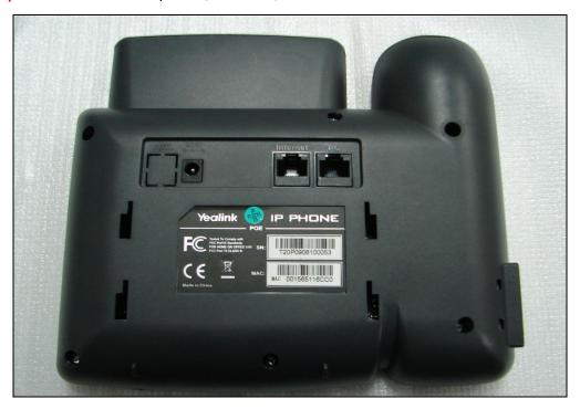
Step2: Loosen 6pcs of screws, open the back shell.
