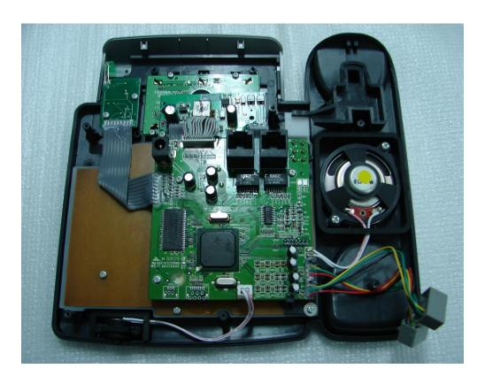
**Step3:** Pull out the male plug of the microphone and the LCD module. Remove 2pcs wires of the speaker with a hot iron.
