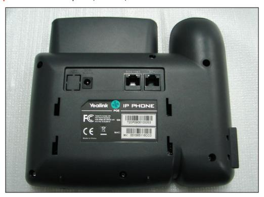
Step2: Loosen 6pcs of screws, open the back shell.
