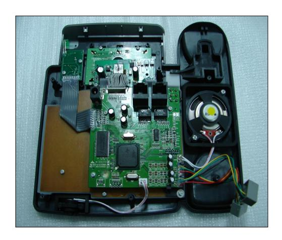
**Step3:** Remove the adhesive with alcohol. Pull out the male plug of the LCD module and microphone.
