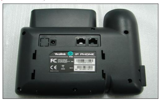
Step2: Loosen 6pcs of screws, open the back shell.
