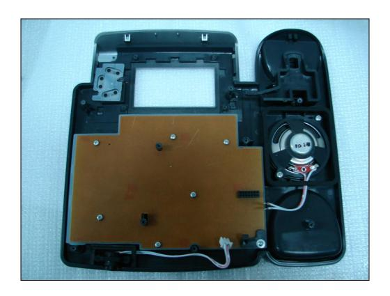
**Step6:** Separate the LCD module from the plastic baffle board and take away the damaged one.
