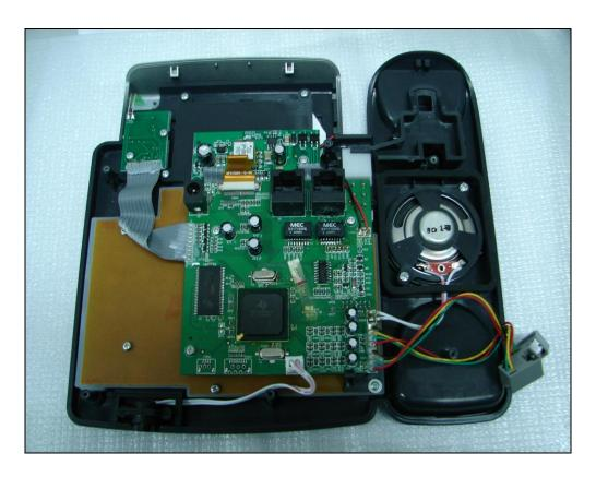
Step3: Remove 2pcs wires of the speaker with a hot iron and the sealing ring. Loosen 2pcs of screws and take away the damaged one.
