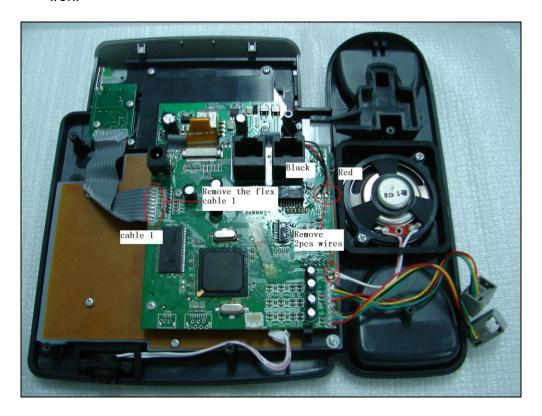
Note: 1. The temperature of hot iron must be less than 350°C;
