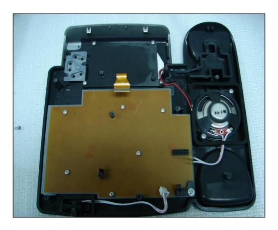
**Step5:** Loosen 4pcs of screws on the LCD module, and take away the plastic baffle board.
