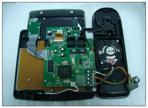
**Step3:** Pull out the male plug of the microphone. Loosen the connector on the direction as shown, and pull out the FPC. Remove the 2pcs wires of LCD backlight and speaker with a hot iron.
