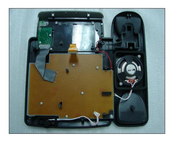
**Step6:** Remove adhesive with alcohol and remove the flex cable 1, cable 2.
