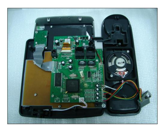
**Step3:** Remove the adhesive with alcohol, and pull out the male plug of the microphone. Loosen the connector on the direction as shown, and pull out the FPC.
