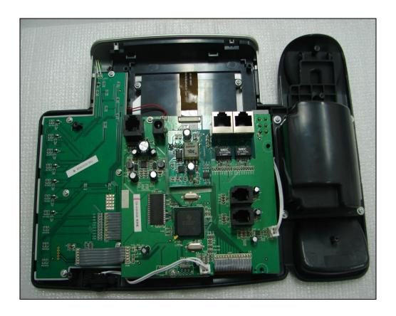
**Step3:** Pull out the plug of the microphone and speaker, loosen the connector of the LCD module on the direction as shown, and pull out the FPC.
