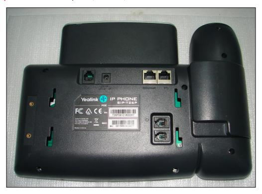
**Step2:** Loosen 7pcs of screws, open the back shell.
