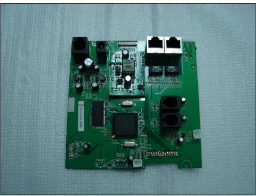
**Step6:** Install the new mainboard in the opposite way following the steps mentioned above.
