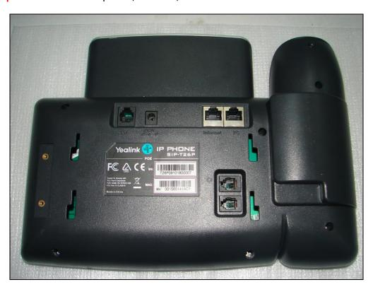
**Step2:** Loosen 7pcs of screws, open the back shell.
