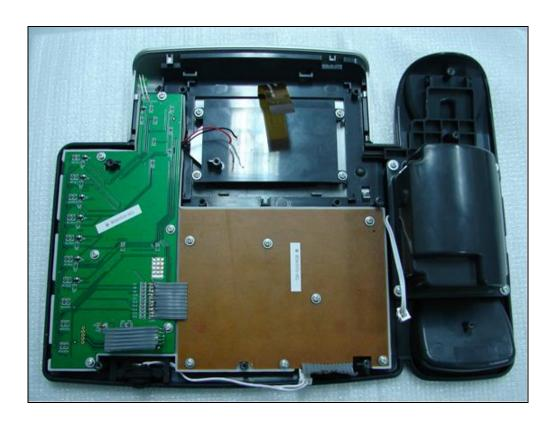
**Step6:** Remove the flex cable 4 with a hot iron. Loosen 7pcs of screws on the keyboard, and take away the damaged one.
