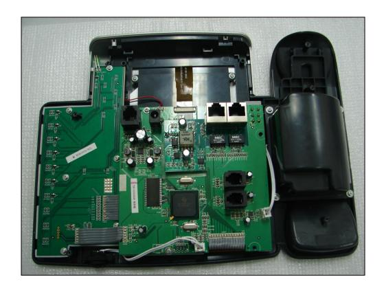
Step3: Pull out the plug of the microphone and speaker, loosen the connector of the LCD module on the direction as shown, and pull out the FPC.
