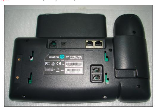
Step2: Loosen 7pcs of screws, open the back shell.
