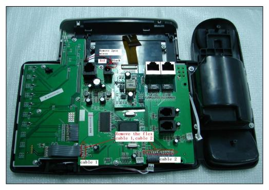
Note: 1. The temperature of hot iron must be less than 350°C;
