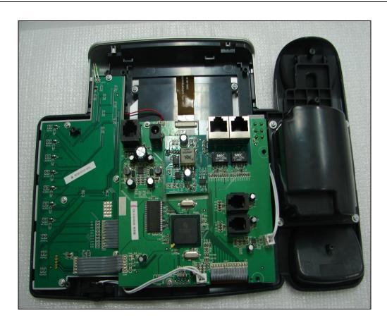
**Step3:** Pull out the plug of the microphone and speaker, loosen the connector of the LCD module on the direction as shown, and pull out the FPC.
