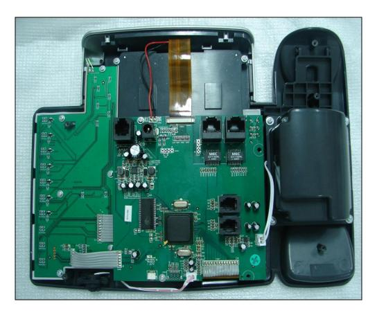
**Step3:** Pull out the male plug of the microphone and speaker, loosen the connector of the LCD module on the direction as shown, and pull out the FPC.
