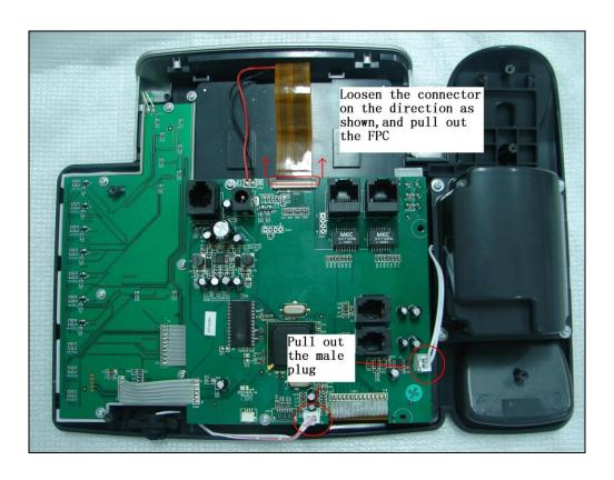
**Step4:** Remove the flex cable 1, cable 2 and the wire of LCD backlight with a hot iron.
