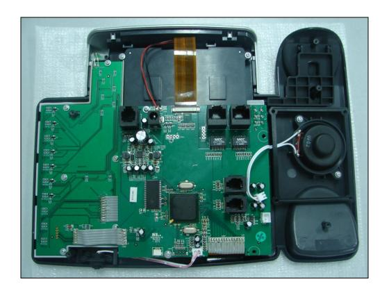
**Step4:** Remove the sealing ring and loosen 2pcs of screws, take away the damaged speaker.
