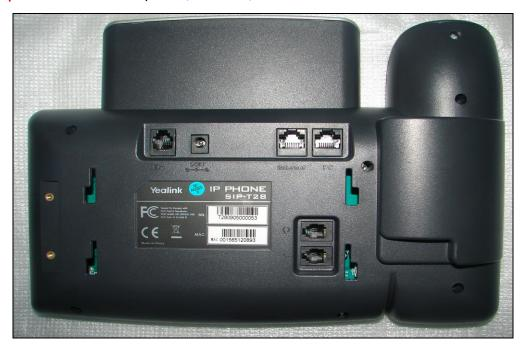
**Step2**: Loosen 7pcs of screws, open the back shell.
