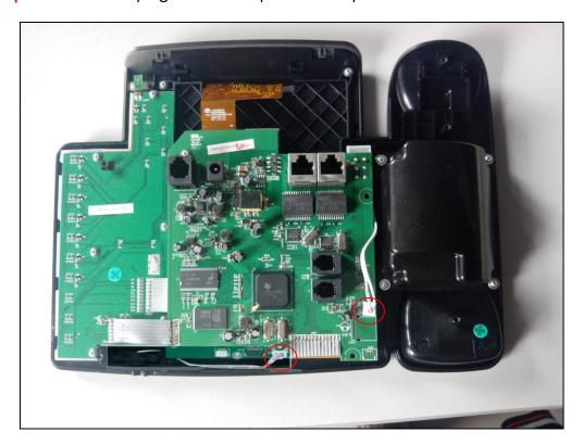
**Step4:** Remove the three flex cables with a soldering iron and the 2pcs of screws on the mainboard. Then remove the LCD FPC cable, take away the mainboard.
