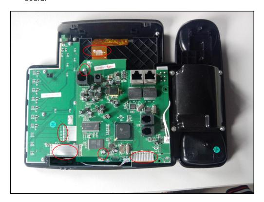
**Step5:** Loosen 7pcs of screws on the keyboard, and take away the damaged one.
