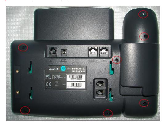
**Step3:** Pull out the speaker cable, loosen 4pcs of screws and open the speaker cavity back shell.
