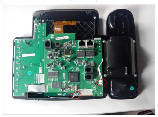
**Step4:** Remove the three flex cables with a soldering iron, and the 2pcs of screws on the mainboard. Then remove the LCD FPC cable, take away the mainboard.
