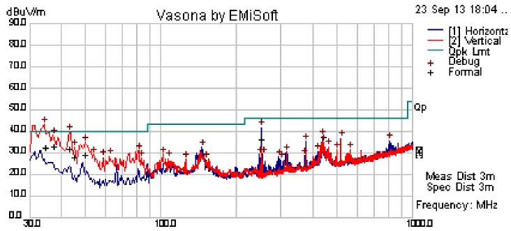
Radiated Emissions Template: 30MHz-1GHz RE Filename: c:\program files\emisoft - vasona\results\FCC 158 2013-09-23-Unit 1.emi
