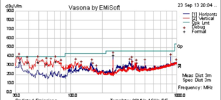
Radiated Emissions Template: 30MHz-1GHz RE Filename: c:\program files\emisoft - vasona\results\FCC 15B 2013-09-23-Unit 2 T-28.emi
