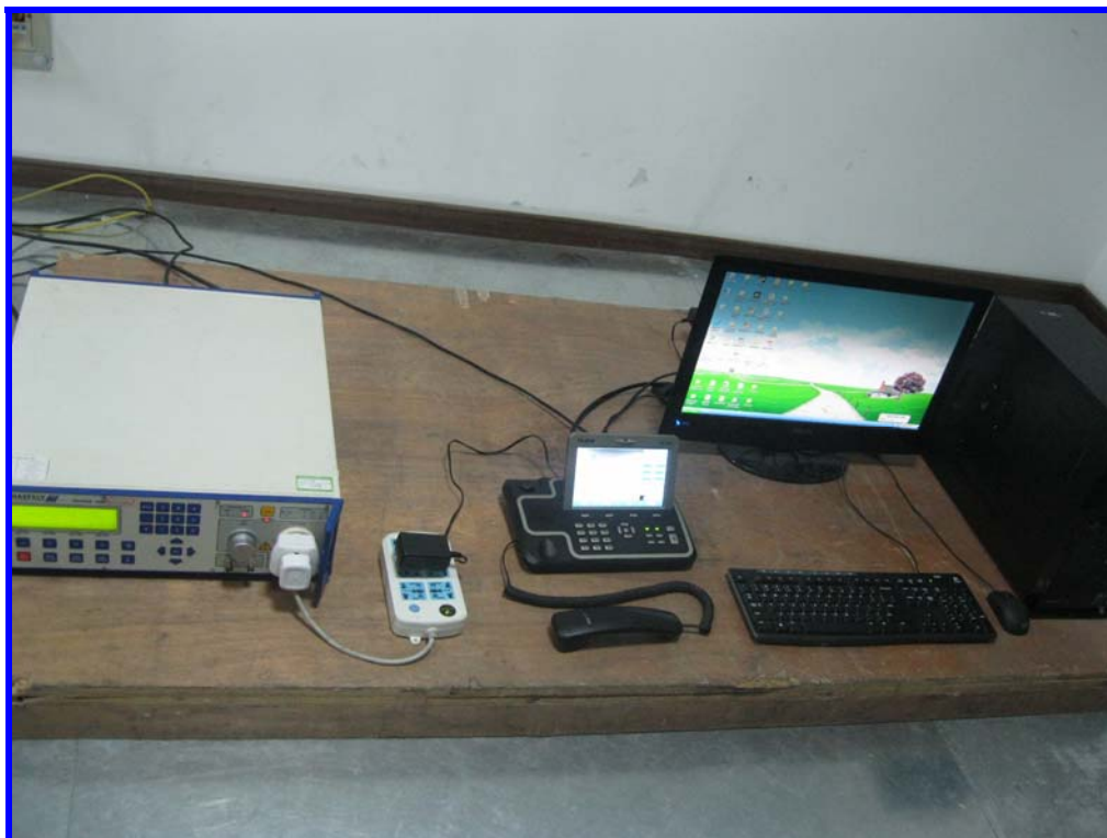
Surge Immunity Test Setup Front View
