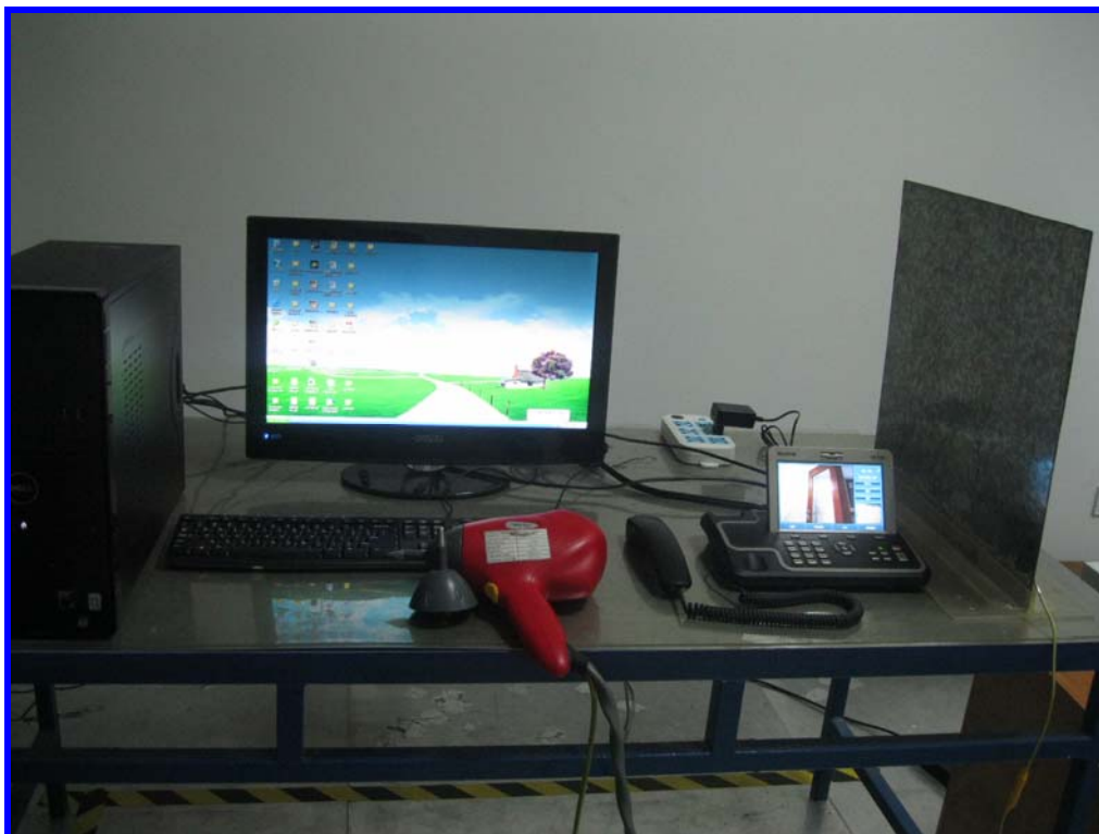
ESD Immunity Test Setup Front View
