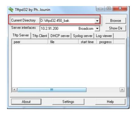
Configure the local IP address in PC. The PC IP address must be configured the value as below. Then the base will get the DECT IP (192.168.0.100) automatically.
