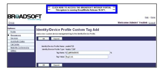
After the above settings, the customizing static tags will only be effectual for the device profile (e.g. yealinkT28).
